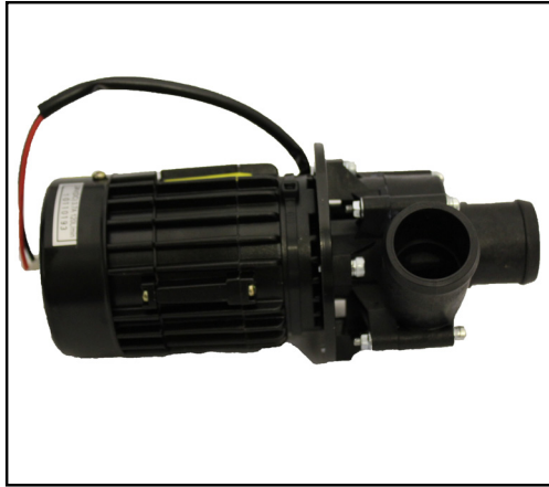
Grayson Reference: MP-1031-005 (Brushless) Circulation Pump Alternative to HP-1515-000 Voltage: 24V Speed: 6,000 litres/hr Weight: 2.55kg or 5.62lbs Inlet/Outlet Ports: 38mm
